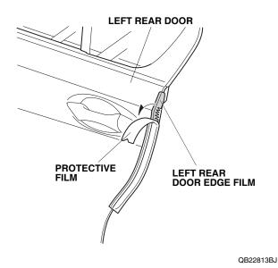
18. Starting from the center and working outward, use your fingers to fold the left rear door edge film around the edge of the door as shown. Move your fingers in one direction only. Attach the door edge film over the seam sealant. Do not damage the door seam sealant.
