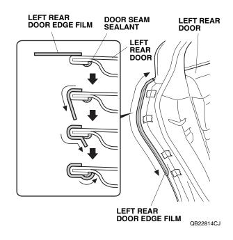
19. Using a shop towel, wipe the excess 3M protective tape application solution from the left rear door edge film. Allow the left rear door edge film to dry thoroughly.
