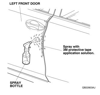
7. Open the left front door. Peel back about 50 mm (2.0 in.) of adhesive backing from the left front door edge film. Align the V-notch in the left front door edge film with the character line on the left front door.
